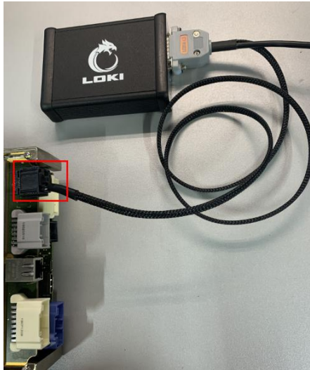
Figure 46. BroadR-Reach port for connection of LOKI to Tesla Model 3
